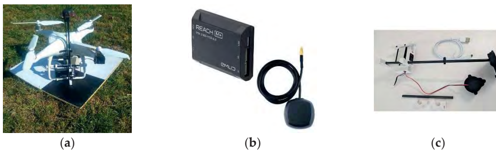
Figure 2. UAV and PPK-GNSS module : (a) Phantom 4 pro ; (b) Emlid Reach M+ and Tallysman antenna; (c) Snap PPK adapter kit for Phantom 4 pro [7]
