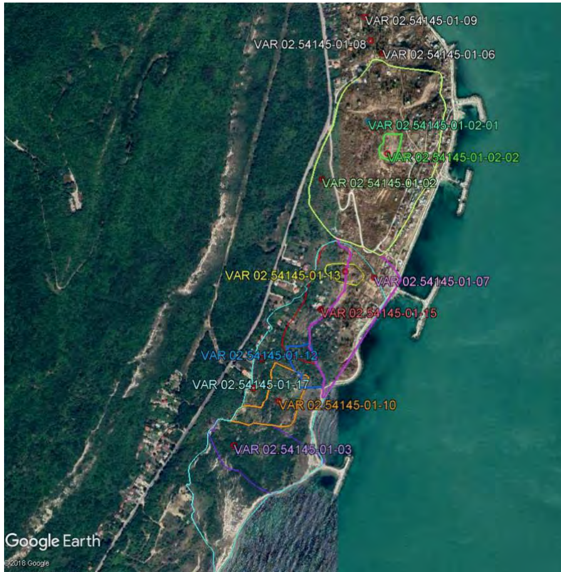
Figure 6. ID codes from MRDPW register and the boundaries of the investigated landslides.
