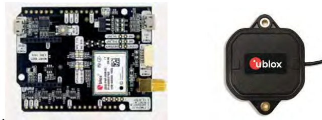
Figure 4. ArduSimple SimpleRTK2B dual frequency RTK application card based on ZED-F9P ($ 200) on the left, multi-band GPS patch antenna on the right ($ 53)
